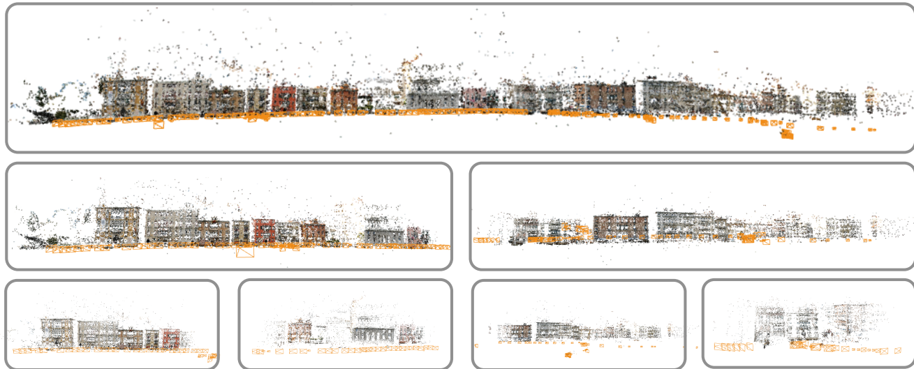
Figure 1. We introduce HyperSfM, a divide-and-conquer approach for Structure from Motion. We represent an SfM problem by a hypergraph which we recursively partition, obtaining a tree of fully-constrained, nonlinear sub-problems. The top three levels are shown above for the "Grand Canal" data-set [1]. After partitioning, computation proceeds from the bottom up, recursively merging submaps.
