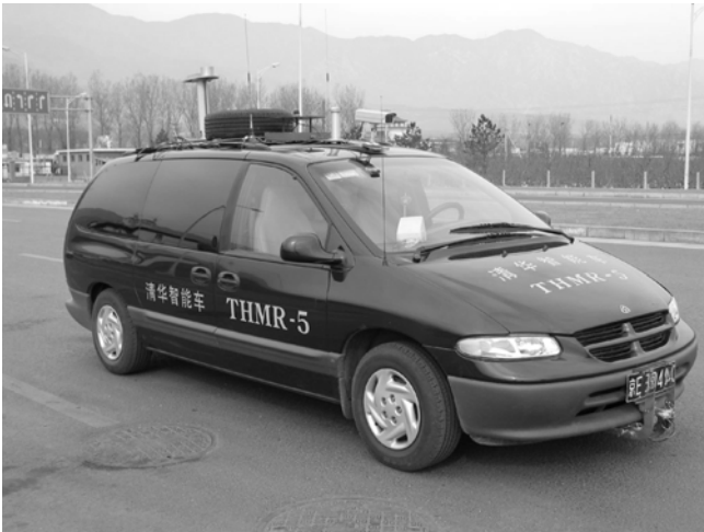
Fig. 1. THMR-V vehicle equipped with CCD camera, GPS, magnetic compass, and optical encoder.
